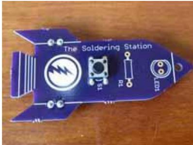
Solder all four pins that are sticking up. The leads are short, so no need to clip them off.
