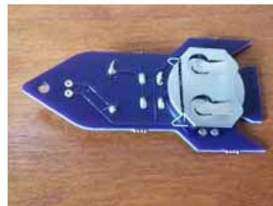
Now solder the two resistor leads and then cut them close to the top of the solder.
